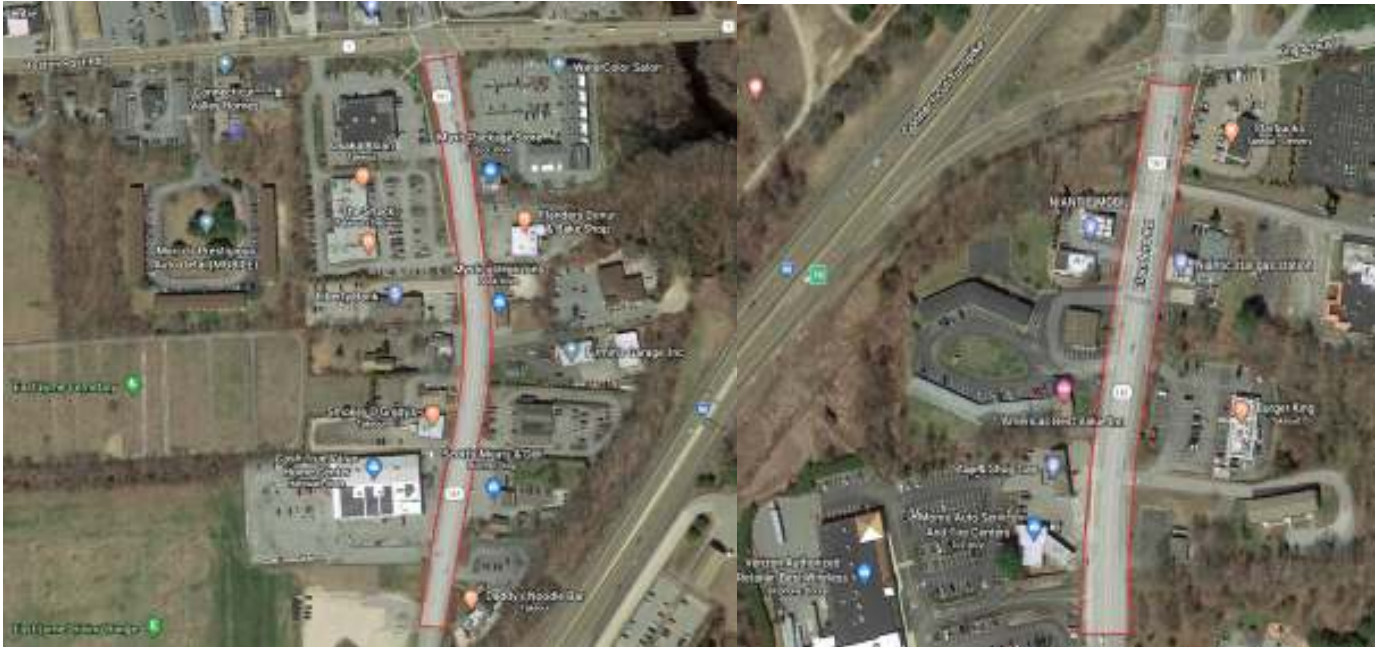
Figure 39 - Recommended Center Turning Lane on Route 161 - North of I-95
