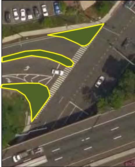
Possible Pedestrian Improvements Ledge Road at Boston Post Road
