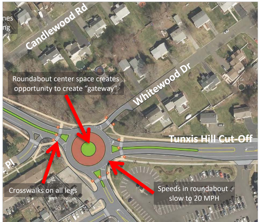
Roundabout concept for the Black Rock Turnpike & Tunxis Hill Cut Off intersection. Source: FHI
