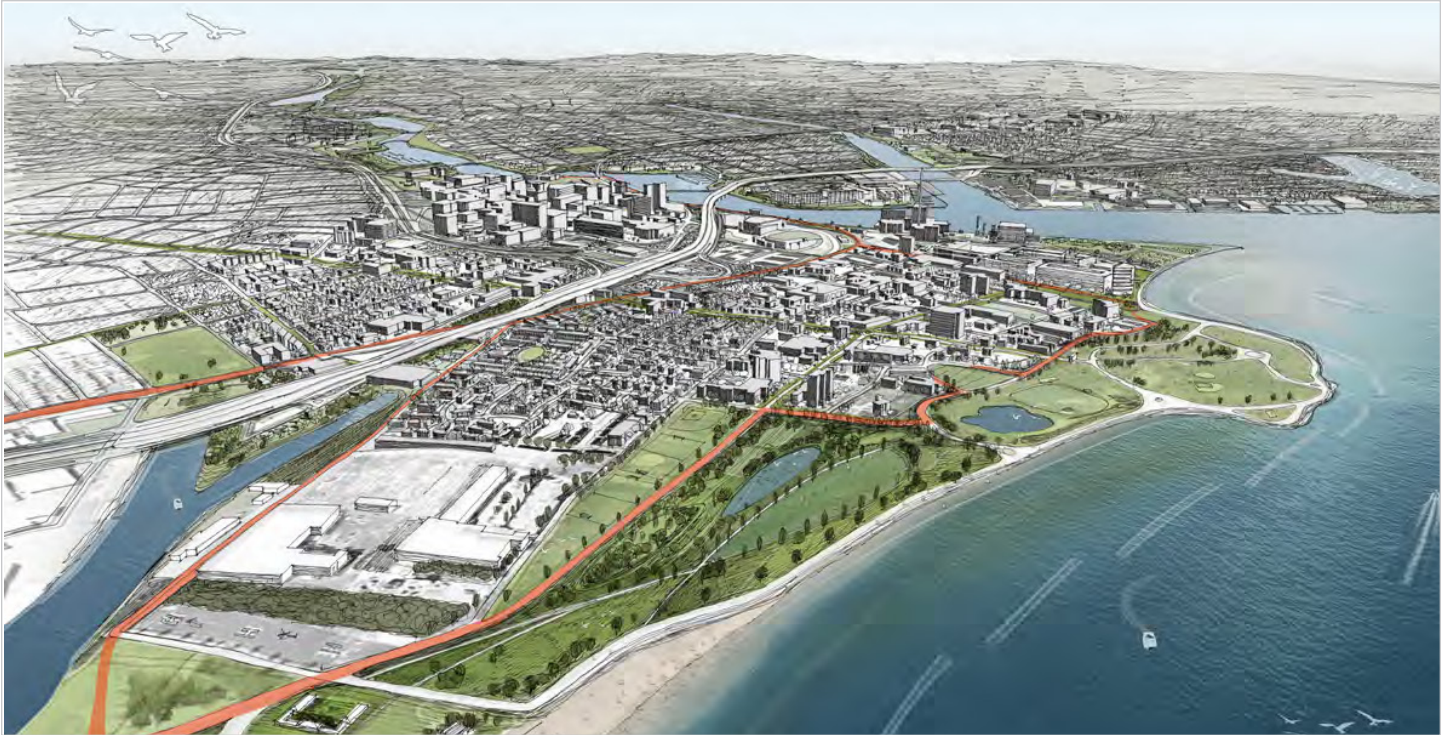
Concept to protect Bridgeport's South End from future floods. The orange lines indicate areas of defense. Source: Resilient Bridgeport.
