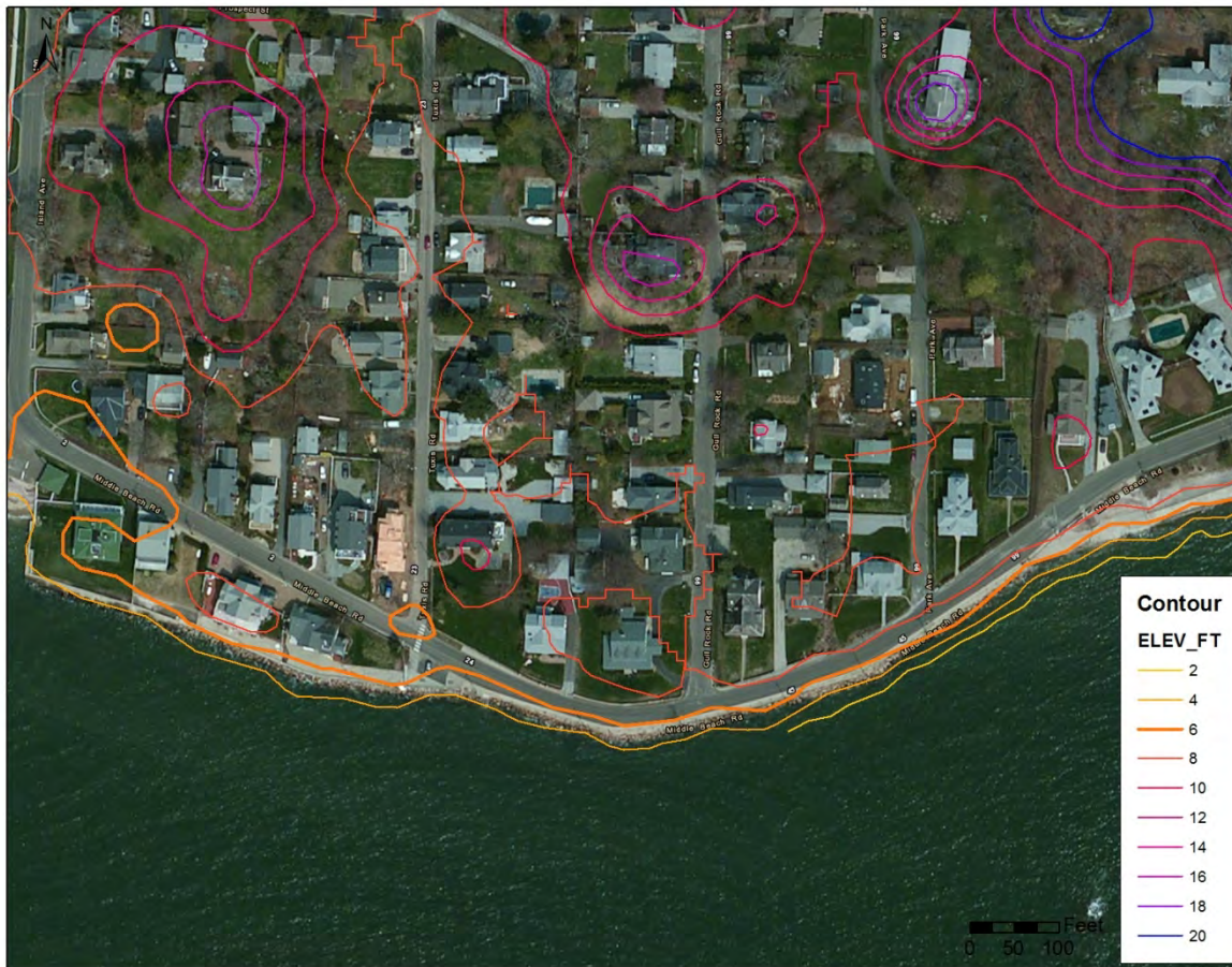
Figure 5 - Topographic Contours Along the Shoreline at Middle Beach Road
