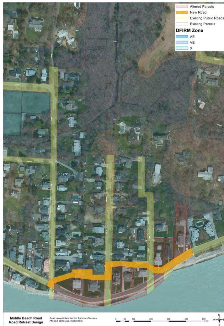
Figure 3 - Abandoning a Stretch of Middle Beach Road and New Road Construction
