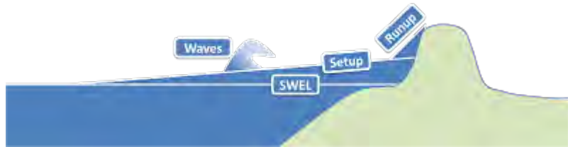
Figure 3: Conceptual representation of stillwater elevation (SWEL), wave setup, and wave runup.
