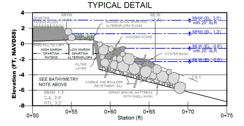
Note: The submerged bank slope and bathymetry is unconfirmed and highly dynamic. Supplemental bathymetric survey is required for final design.
