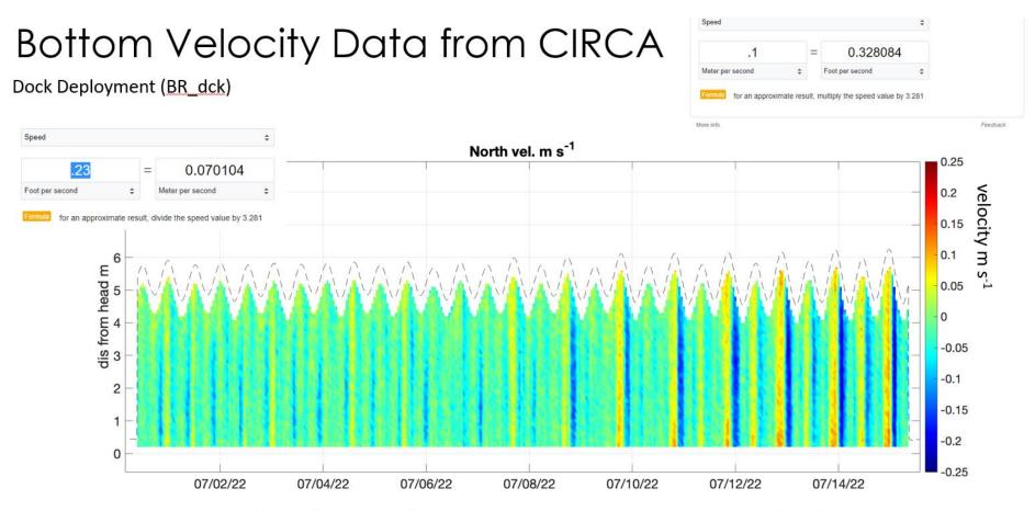
Distance from head of the instrument. The ADCP sits ~ 10 cm above the bed. Surface is marked in dashed black.
