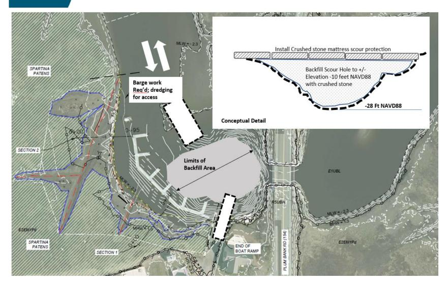
Figure 5: Supplemental Construction Conceptual Detail – Backfill and Scour Protection of Existing Scour Hole
